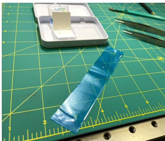
Fig.3: Exfoliated 2D hexagonal Boron Nitride (hBN) on Nitto SPV224 PVC Vinyl tape.
