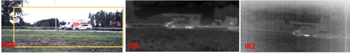
Fig. 1. Sample triplet of collected images consisting of RGB, wide band (8-14  $\mu\text{m}$ ) LWIR IR1 image, and 9.5  $\mu\text{m}$  (0.5  $\mu\text{m}$  band) IR2 image. Note hot brakes and muffler under the car on the IR images.
