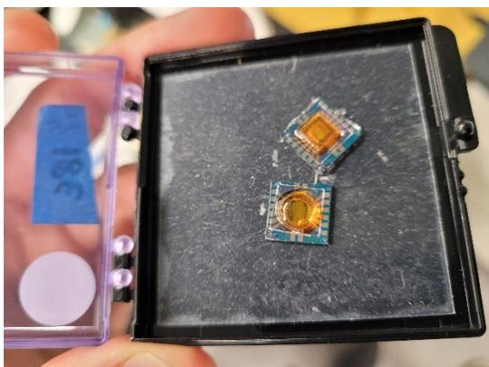
Fig.2: Sealed Electrolytes on Graphene Devices. Graphene Field-Effect Transistors Acquired Commercially from Graphenea, Consists of 2x6 Array of 100um x 100um Graphene Transistors with an Unpassivated Gold Side-Gate. Sealed with NOA71 Epoxy
