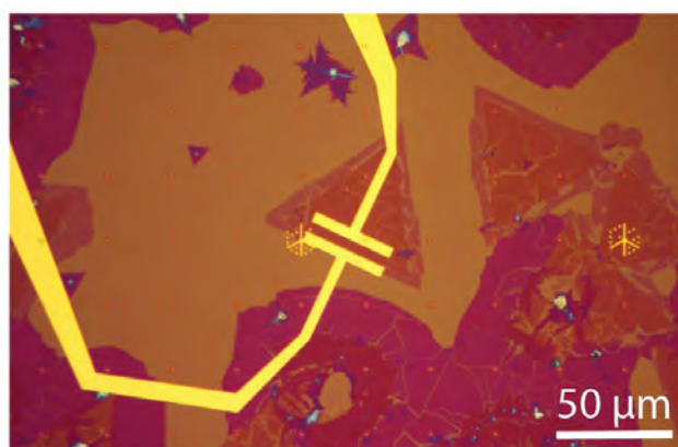
Fig.4 Optical microscope image of an automatically fabricated two-terminal device with a 4 \mu\text{m} channel across the interface between \text{MoSe}_2 and \text{WSe}_2 .
