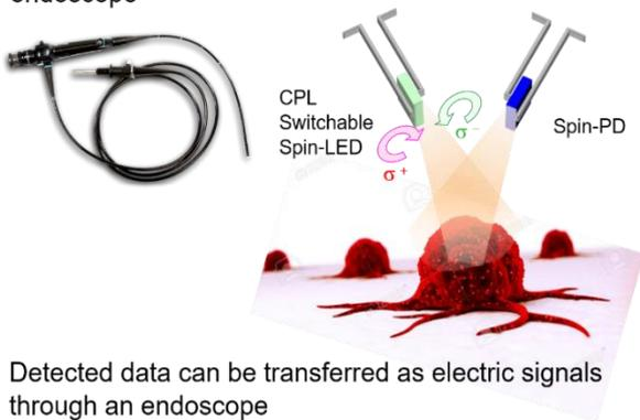
Fig.1: Schematic illustration of in vivo detection of tumor tissues using a spin-LED, a CP emitter, and a spin-PD, a CP detector. These devices are supposed to be integrated into an endoscope that is shown on left- top side of the figure.
